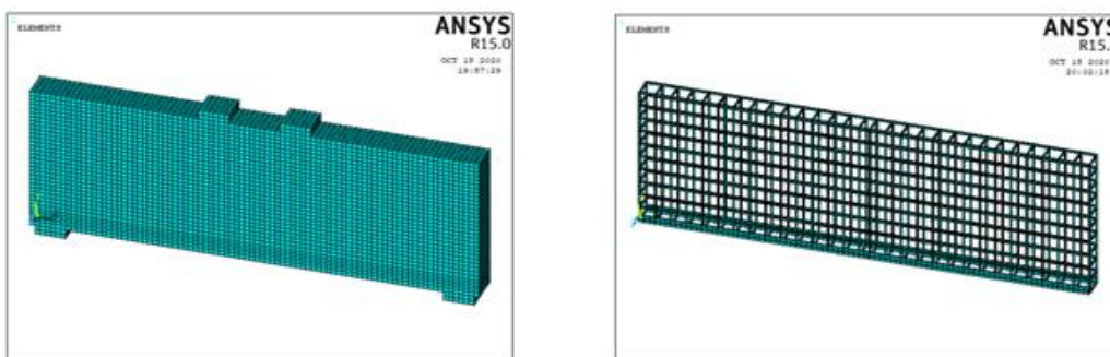
(a) Concrete elements (Solid 65)
